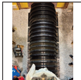
Figure 8: HydroChain S-29B Chambers Assembled in the Soil Box
