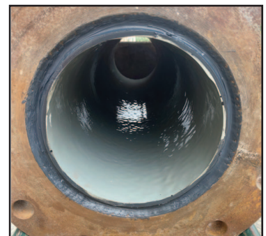
Figure 4: External Buckling Test Assembly (Left) and Inside View of the Pipe Sample Sealed at both Ends (Right)
