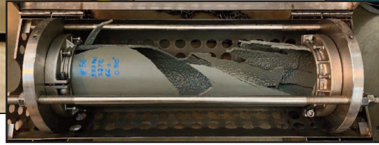
Figure 6: Burst Pipe Sample
