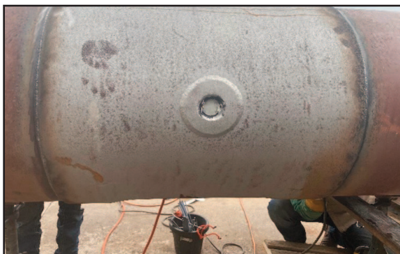
Figure 3: Hole-Spanning Testing Pipe Sample
