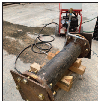
Figure 4: External Buckling Test Assembly (Left) and Inside View of the Pipe Sample Sealed at both Ends (Right)
